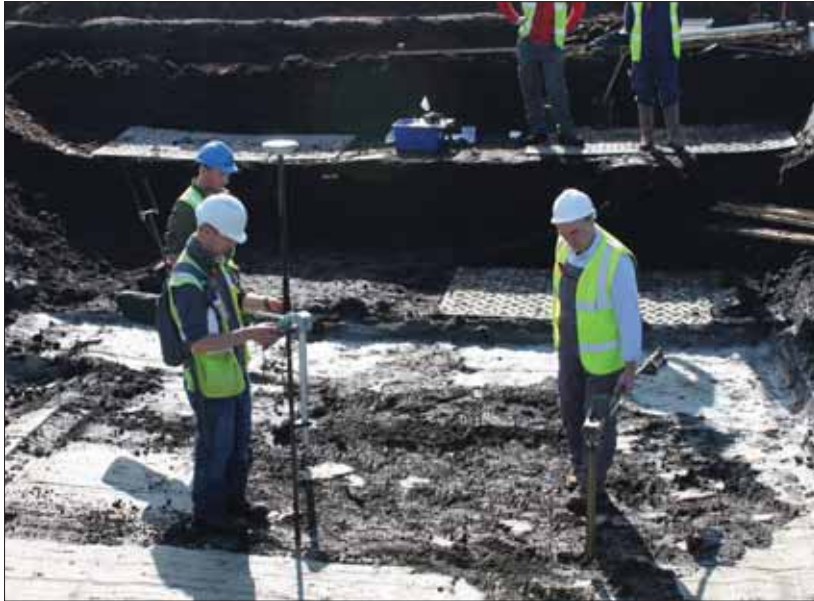
Plate 13: DGPS locating of the impact crater and use of magnetometer to locate the engine block
